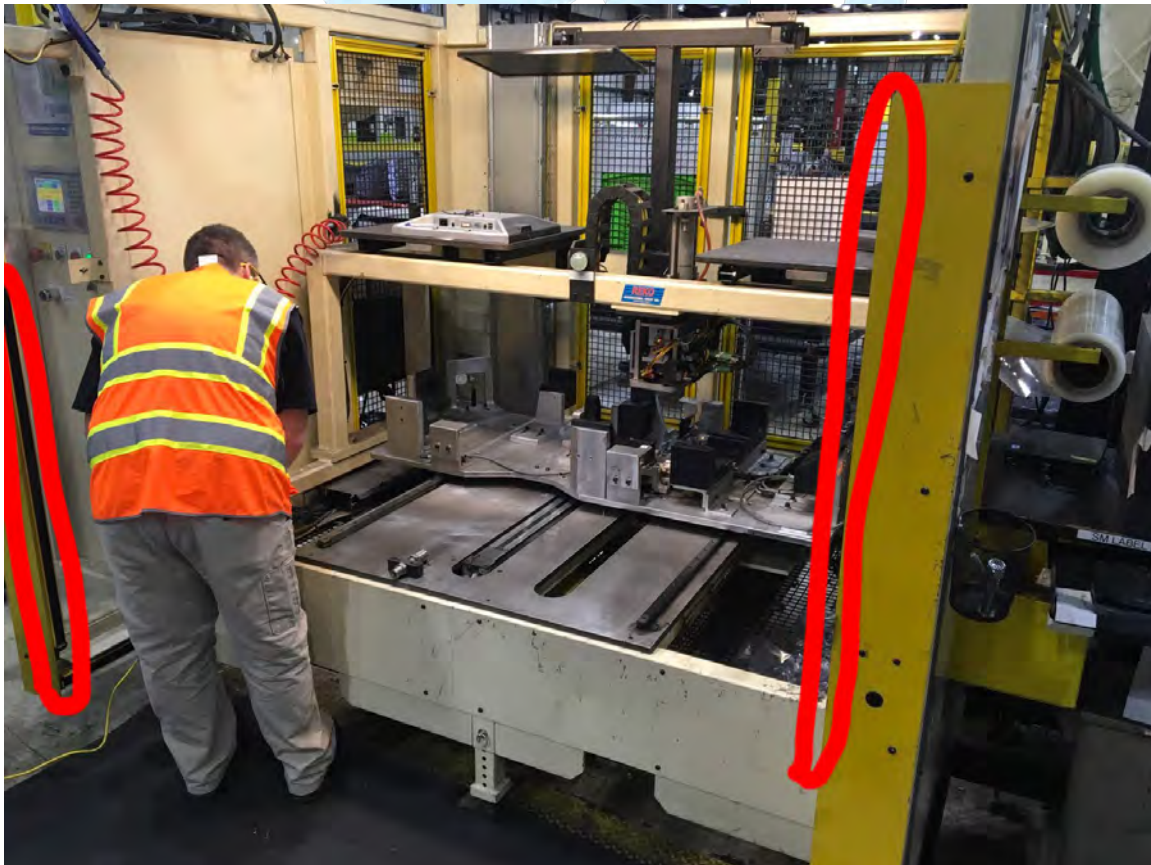
Machine overview. Light Curtains too close. Move to safe distance or improve stopping performance of Slide table.
